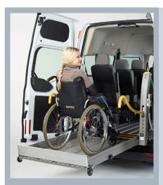
Worldwide unique design due to the specially manufactured aluminium profile lifting arms.
